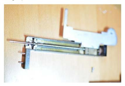
The Y movement is simply a pinion that rolls against the geared rail in the stage. I cleaned and lubricated both parts with standard mineral oil:
