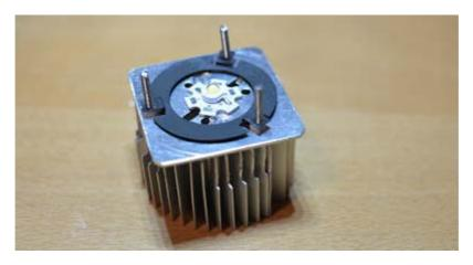
Put it all together, inside the microscope base (mounted the LED + heatsink, the step-down converter PCB, the DC connector, and the potentiometer, in the place where the original one would go).
