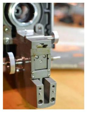
The bottom rectangular part held together by four screws, have behind two springs. After removing the screws, to avoid having to remove the springs (and later having the challenging task of placing these again), I simply moved the part to the bottom, keeping the springs under tension:
