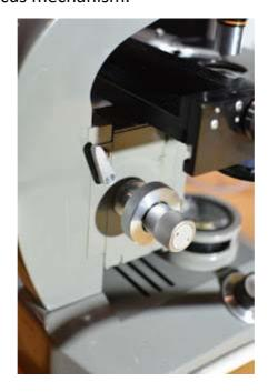
To remove the fine focus, I used a set of pliers of the type used for installing retaining rings. docking its pins to the pair of holes in the face of the fine focus knob:
