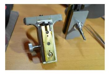
With the fine focus body removed, it was now a matter of cleaning very well all the dampening grease bearing parts, and apply fresh grease (I used standard lithium-based grease, which should be ok, even though there are more specialized greases). The cleanup was a particularly time-consuming task, as the grease was persistently attached to the metal surfaces.
