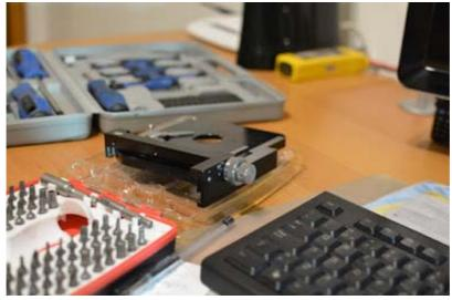
A cover in the top of the assembly must also be removed in order to allow the focus assembly to slide out of the microscope body:
