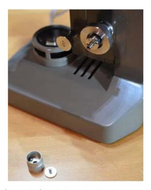
This exposed the fine focus shaft and the cylindrical part populated with 5 screws in different areas of the part (from the parts diagram, parts AA 233700 and AA 750800, from left and right side of the microscope, respectively).
