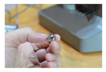
This part has an O-ring which is in contact with the fine focus shaft. Apparently it is made of nylon or eventually Teflon. This is one of the very few plastic parts I could find in this microscope.
