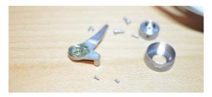
As seen above I have also removed the slide retainer tweezer to also clean and lubricate with grease.
