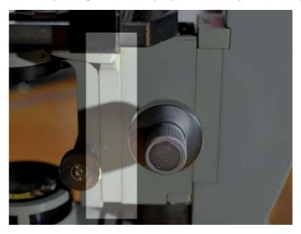
So I found that there was a lever that would cause this intermediate part (to which the specimen stage actually is attached) to move, based on the position of the disc. The lever is hidden behind the disc and the pinions, so that it was difficult to identify it at first. As it moves, it pushes against the long, adjustable screw that can be seen on the photo, causing the assembly to be moved up or down:
