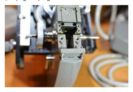
In order to remove the focus assembly, I had to remove the specimen stage by removing the four Allen screws that keep it attached:
