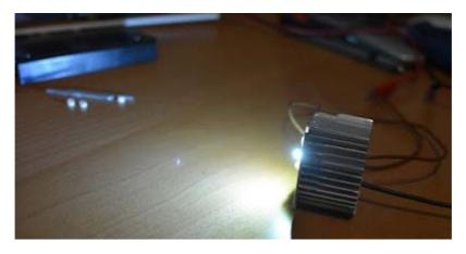
Made some tests with the step-down converter, limiting the current to 500 mA (below the rated 700 mA but more than enough for the lighting requirements), and replacing the on-board multiturn pot by a 500 Ohm panel potentiometer and
