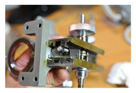
So, at this point the problem seemed obvious: the dampening grease aged and became sticky (as in most joints in this microscope), and the disc mechanism was no longer able to move the fine focus body. The short travel length the fine focus rail has to move clearly must have contributed to cause the part to become stuck.
