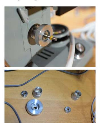
Then in the left side knob, I got stuck with the coarse focus knob retaining bolt. Unlike the right side one, this has the two holes for removal with a special wrench.
