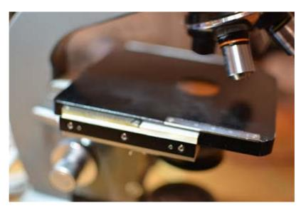
The first thing to remove are the knobs. An Allen and a Philips key are sufficient to remove the two knobs:
