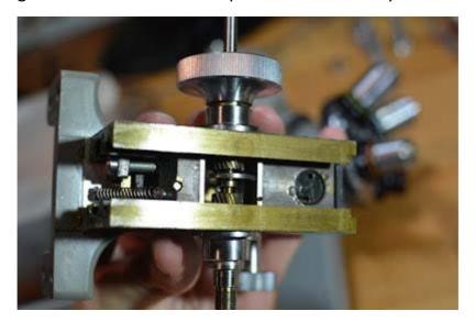
At this point I still did not understand how the fine focus mechanism worked. There was indeed a disc that would move to the left or right as I would turn the fine focus shaft, but I could not see any relationship between that happening and the moving of the focus assembly.
