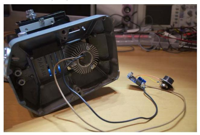
machined an aluminium disc to provide the necessary width for fitting a DC connector in the hole where originally the thick mains cable would pass through:
