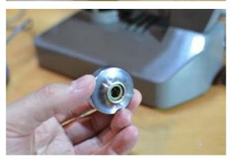
Later I found that I could control the friction of the fine focus knob by adjusting the screws in the bearing removed right after the fine focus knob:
