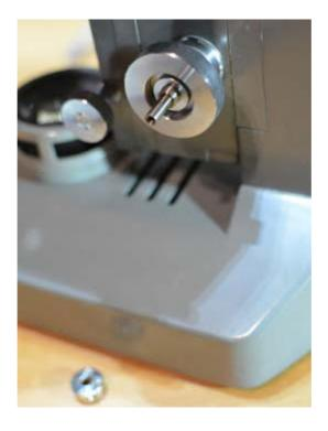
For removing it, one must turn the coarse focus knob counter-clockwise, while keeping the coarse focus knob for the other side fixed. After that, the coarse focus knob can just be pulled off:
