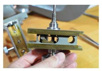
Applying grease to the surfaces. In respect to the pinions and toothed rails, I used standard lubricant oil:
