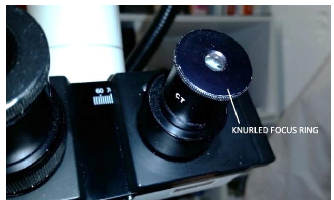
Figure 4 – Adjust knurled focus ring to focus the image
