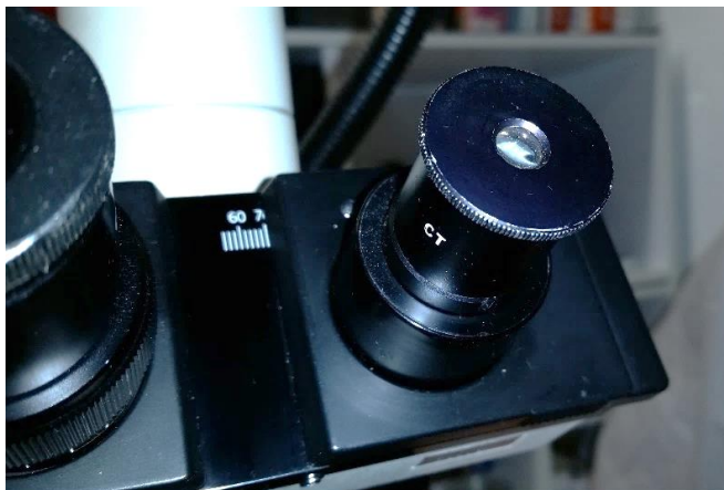
Figure 2 – Replace right eyepiece with phase telescope
