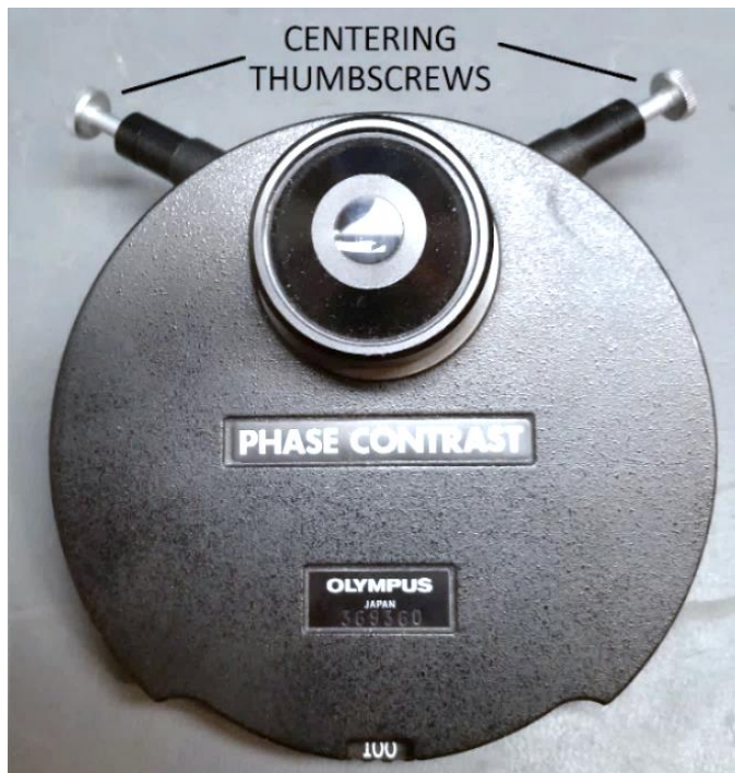
Figure 6 – Centering screws of BH2-PC/PCD condenser
