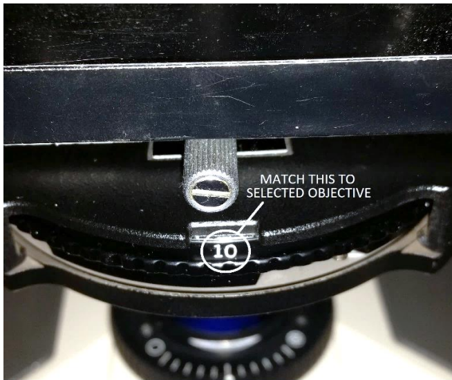
Figure 1 – Set condenser dial to match the objective
