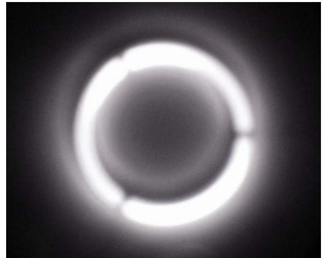
Figure 3 – Phase telescope improperly focused
