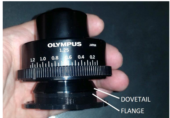
Figure 12 – BH2-OBL installed in the condenser (BH2-CD)
